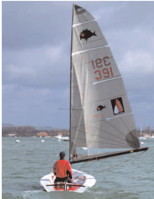
Left The laminate Kevlar sail reflects Red Eye's development of Phantom sails.
