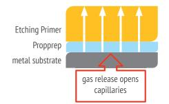
It is this process which relies on the re-coat timing window being strictly followed to ensure excellent product performance (see application video). When the **Clear Coat** is applied it soaks in to these holes, binding to the primer coats as well as the metal substrate.
